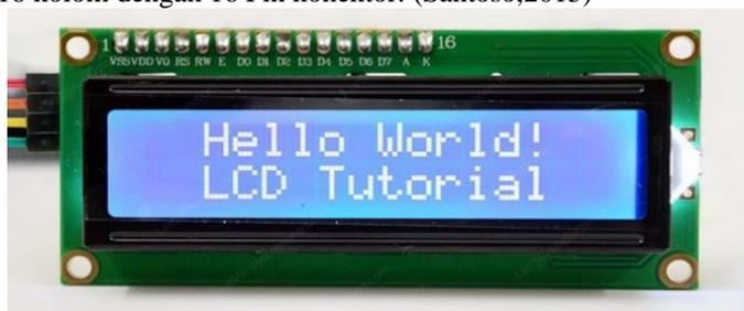
**Gambar 4.** Liquid Crystal I2C (LCD I2C)
