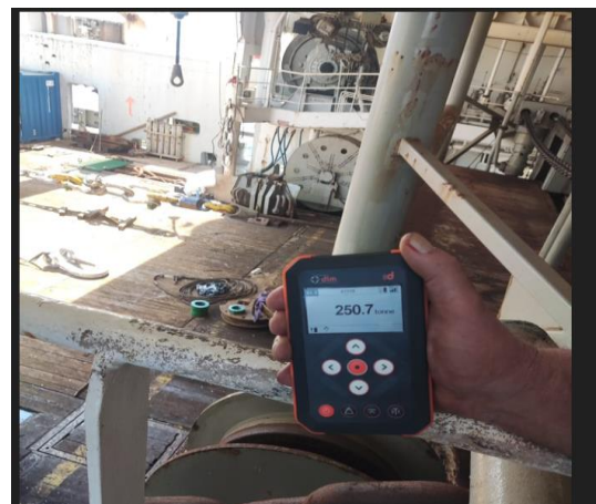
Figure 6. Portable Load Cell
