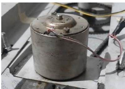
Gambar 4. Generator DC 40 W
